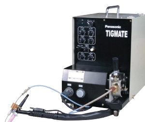
YJ-1052THGG Automatic wire filling device
